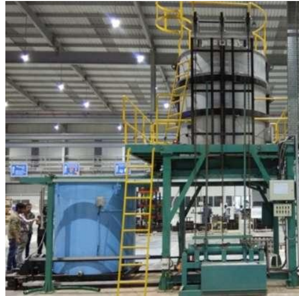
T6 HEAT TRATEMENT FURNACE
