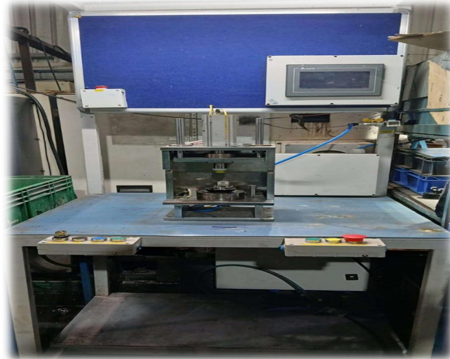
Leak test; Cosmo /ATEQ equipment 70 to 130 Pascal @ 5 bar
