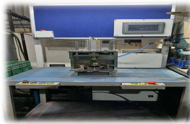
AIR LEAK TESTING MACHINE
