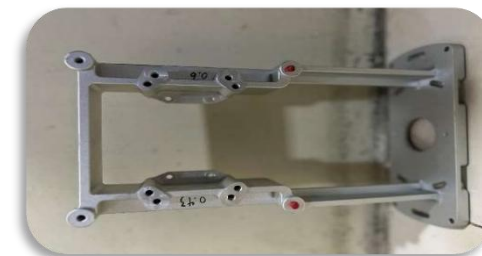
Telecom – 5G Tower OT base casting
